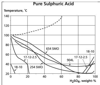
Isocorrosion diagram, 0.1 mm/year, for austenitic stainless steels in naturally aerated sulphuric acid of chemical purity. Broken-line curve represents the boiling point.
